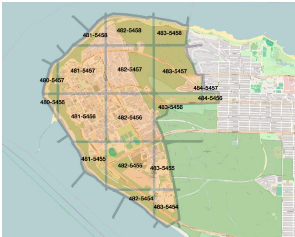
Figure 2. Range of LiDAR data for UBC Vancouver campus with specific area number. Data covers the geographic bounding between -123.261^{\circ}\text{W} to -123.191^{\circ}\text{W} and 49.2793^{\circ}\text{N} to 49.2328^{\circ}\text{N} . This LiDAR coverage map is projected in NAD 1983 UTM Zone 10N and sourced from Campus and Community Planning (2015).
