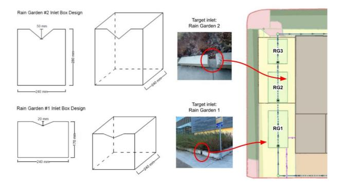
Figure 6. Weir box design with dimensions for both RG 1 & 2.
