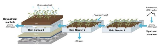
*Figure 1.* Simplified illustration of the study site's system of three RGs. Blue arrows represent the flow of water. After passing through the downstream manhole, water is then directed to a detention tank and drained into existing storm sewer infrastructure as part of the North Catchment, which eventually discharges into the ocean.
