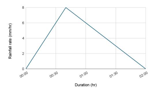
*Figure 11.* Sample design storm for a 2y - 2hr storm event using the triangular method. Rainfall rate (mm/hr) in the hyetograph denotes intensity.
