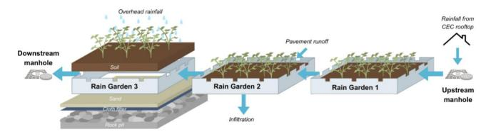
*Figure 5.* Simplified illustration of the study site's system of three RGs. Blue arrows represent the flow of water. After passing through the downstream manhole, water is then directed to a detention tank and drained into existing storm sewer infrastructure as part of the North Catchment, which eventually discharges into the ocean.
