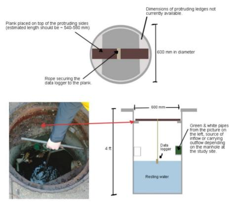
Figure 7. Measurement for the diameter of manhole and planks set up for hanging the water level loggers. Manhole inflow and outflow had the same size of the hole.
