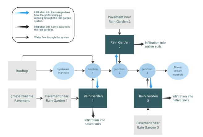
*Figure 10.* Flowchart mapping out the progression of water through the CEC RG system. (Im)permeable pavement represents a permeable pavement which has not been maintained since installation and assumed to have lost most of its function.
