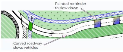
Figure 7: Roundabout Design Safety Features
