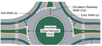
Figure 2: Key Roundabout Dimensions
