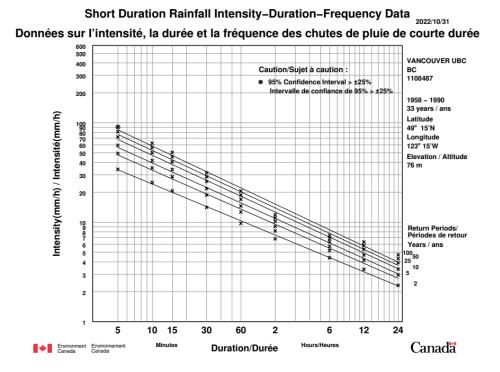
Figure 31: Short Duration Rainfall Intensity - Duration - Frequency Data
