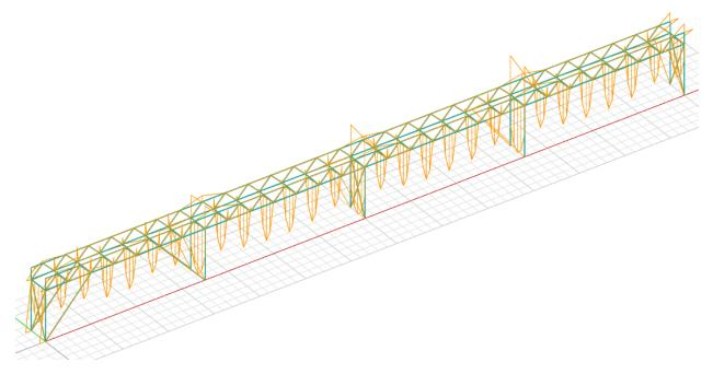
Figure 30: Overpass Case 5 X Axis Bending Demands
