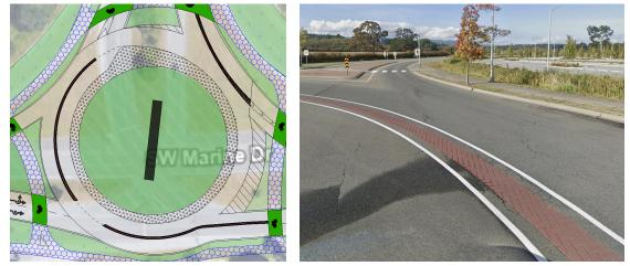
Figure 8 / 9: Roundabout Design / Example of Physical Barrier within Turbo Roundabout at Electra Boulevard and Willingdon Road, North Saanich, BC
