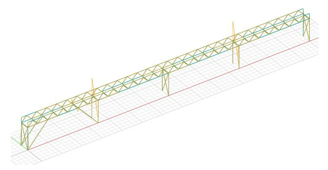
Figure 27: Overpass Case 5 Y Axis Bending Demands
