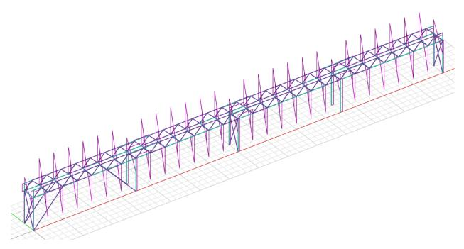
Figure 29: Overpass Case 5 X Axis Shear Demands
