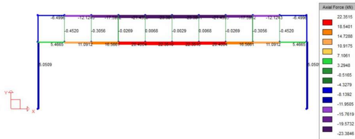
Figure 18: Axial force analysis for each member
