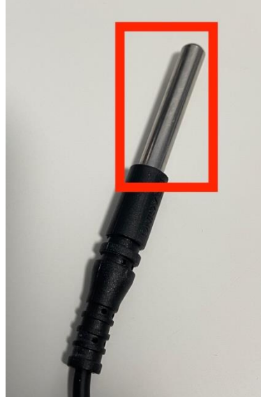
Figure 8: Make sure the metal tip of the temperature probe is touching the window surface.
