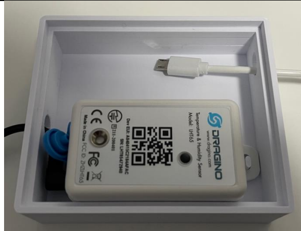
Figure 47: Pass through the micro USB cable from the other hole on the side of the case.
