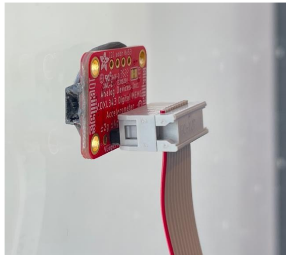
Figure 6: Make sure the accelerometer board is as parallel to the window panel as possible.
