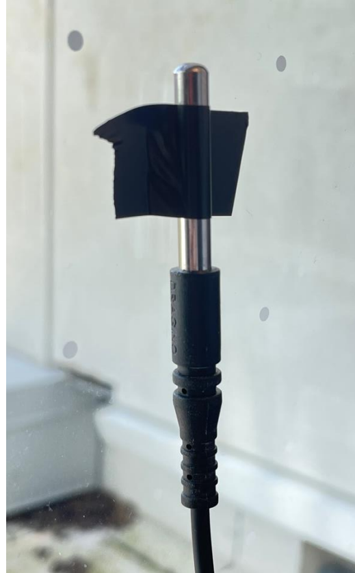
Figure 9: Attach the temperature probe to the window panel with electrical tape.
