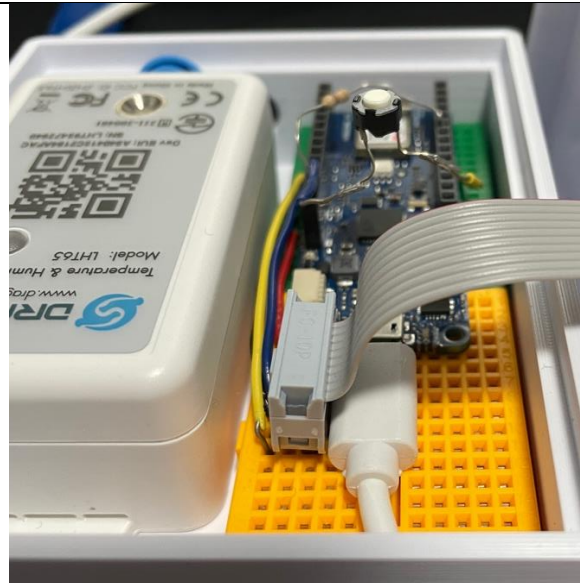
Figure 49: Connect the ribbon cable connector to the pin header on breadboard.
