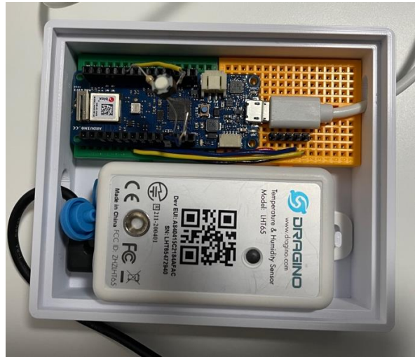
Figure 48: Arduino assembly placed inside the case.
