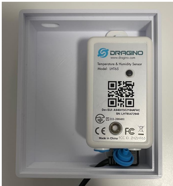
Figure 45: Dragino sensor placed inside the case.
