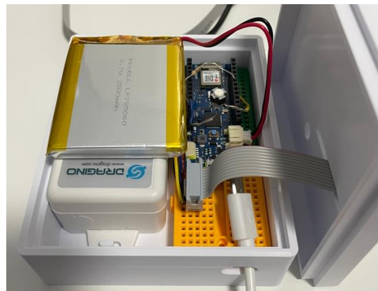
Figure 15: Leave the lid off when powered with battery.
