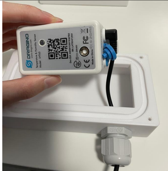
Figure 56: Connect the end of the temperature probe cable to the Dragino sensor.
