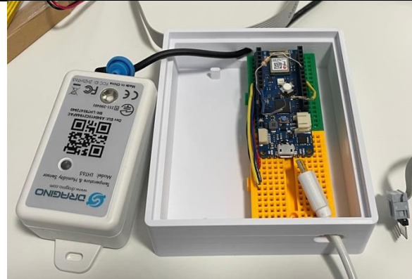
Figure 13: Remove the Dragino Sensor, unplug the ribbon cable, unplug the USB cable, and move the breadboard temporarily.
