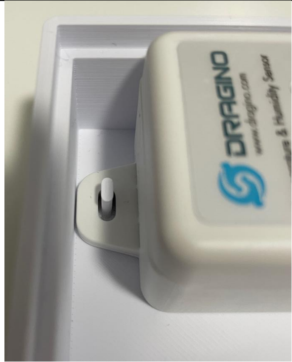
Figure 46: Align the Dragino sensor with the "hook".
