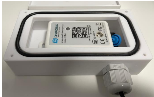
Figure 61: O-ring in the groove.
