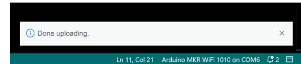
Figure 79: It will say “Done uploading.” once the code is successfully uploaded to the Arduino.
