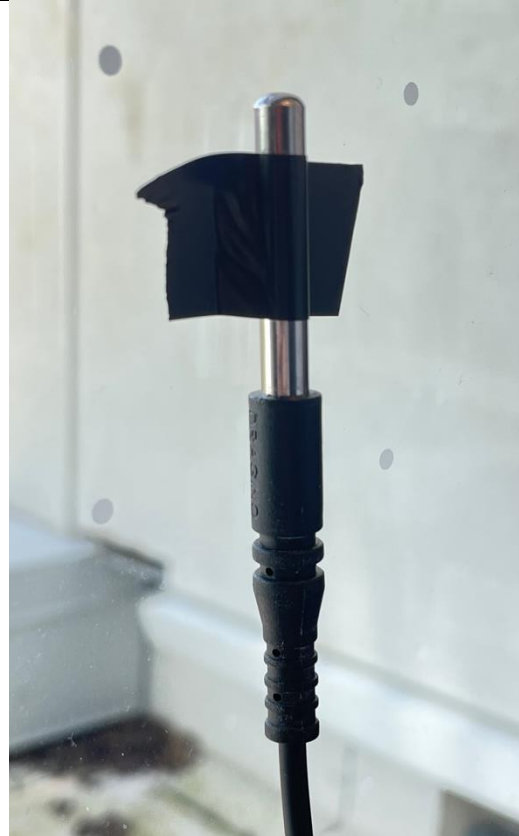
Figure 7: Attach the temperature probe to the window panel with electrical tape.
