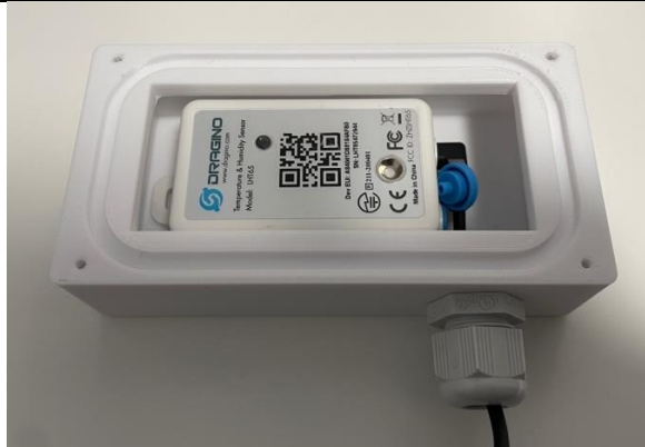
Figure 57: Place the Dragino sensor inside the case.
