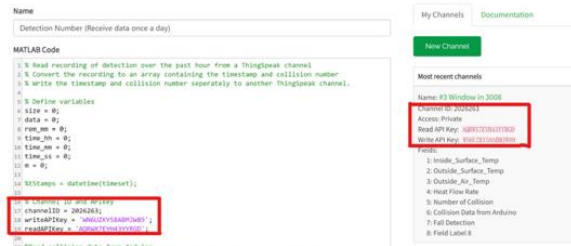
Figure 113: Make sure the channel ID, "write" and/or "read" API Key in the code match with the values on the right-hand side.
