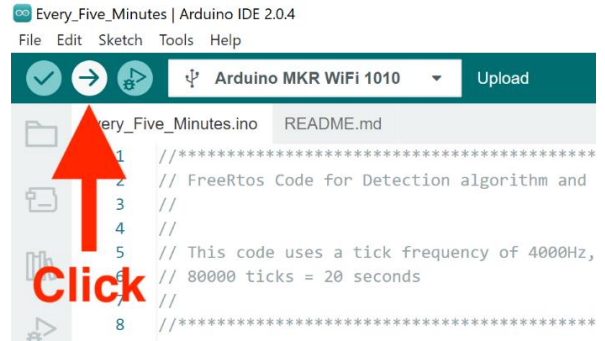
Figure 77: Click the “Upload” button to upload the code to the Arduino.
