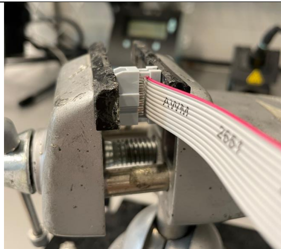
Figure 43: The connector can be clamped using a vise.
