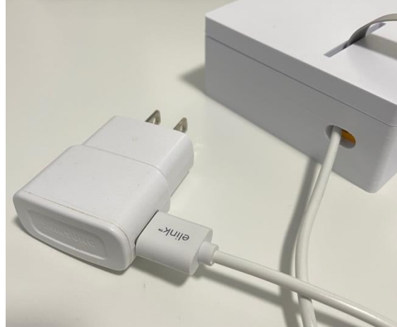
Figure 10: Connect the USB cable to the power adapter.
