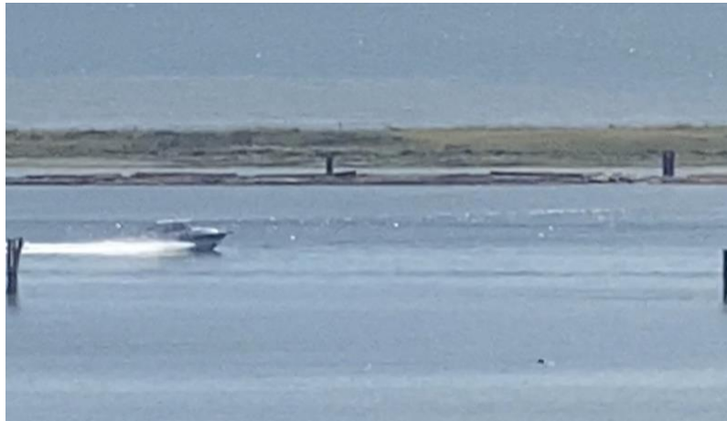
Figure 17. Screenshot taken from a video filming boat passage as part of Observation 1, showing the narrow river and posts used to estimate the speed of vessels based on the time it took to clear the area compared to available speed from AIS vessels.
