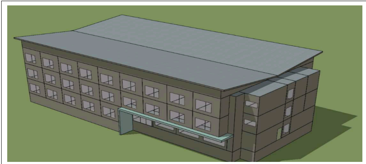
Figure 23- showing the Schematic Design on South-facing wall and small solar shading overhang on the entrance Focal Engineering, (Mar 2018)
